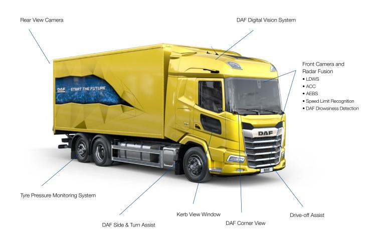
From July 2024, all newly registered trucks in the EU must comply with the new General Safety Regulation (GSR), Package 1. The objective of the GSR is to halve the number of fatal accidents and serious injuries by 2030, and further reduce them to zero by 2050. At DAF, safety is our number one priority, and is already integrated into New Generation DAF trucks from front grille to back bumper. Every model produced for the EU in 2024 will fully comply with Package 1 of the GSR.
